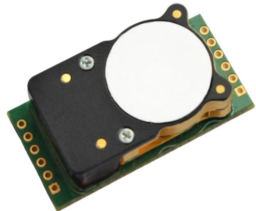
The length of time the light source is active is also a major contributor to how much power is consumed by the sensor. The light source in a CO<sub>2</sub> sensor can be run continuously or pulsed to minimise overall power consumption.
