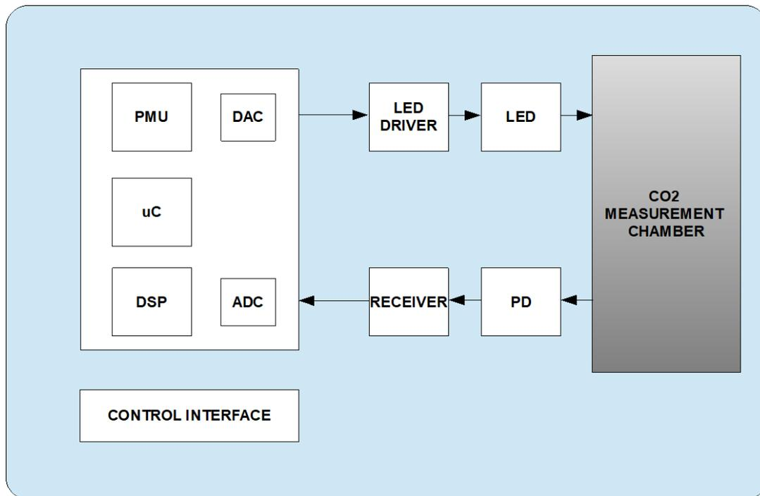
**Figure 1: Block diagram of typical GSS solid-state LED NDIR sensor**
