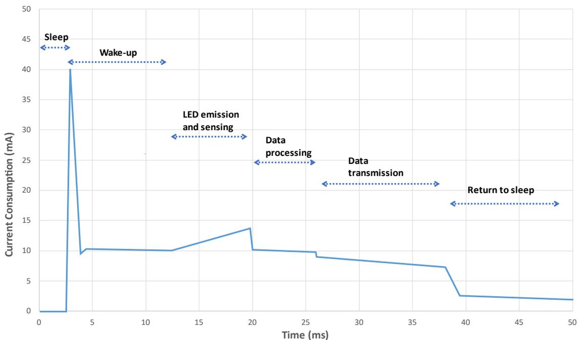
**Figure 3: CozIR®-LP2 typical current consumption profile over 50ms**
