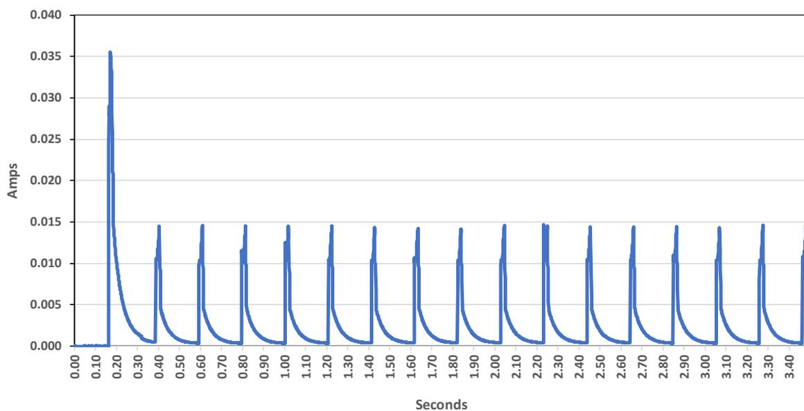
**Figure 5: CozIR®-Blink current profile example showing 16 measurements to produce a single averaged CO<sub>2</sub> reading.**
