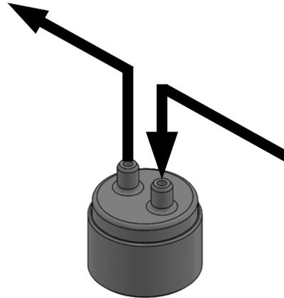
The gas flow can be derived from a sample bleed from a high pressure system, or from a pump that is used to induce flow. Ideally, there should be a match between the required gas sampling speed and the gas flow rate.
