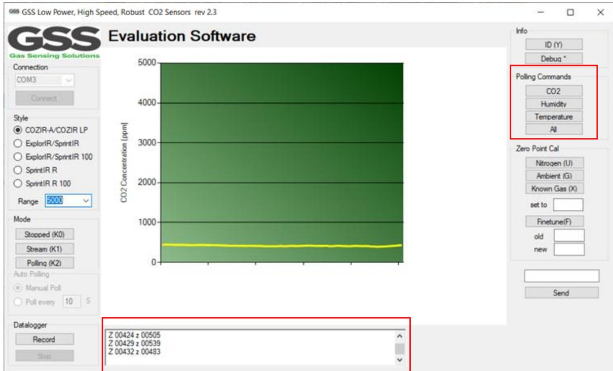
Depending on the sensor type, various parameters can be output as a single string of data in the dialogue box. If a temperature or humidity sensor is fitted, the dialogue box will show the relevant data fields depending on user requirements.
