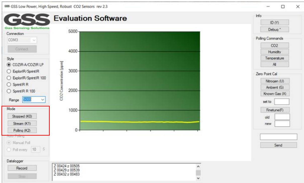
The software interface replicates the UART controls of the sensor. For full details of the functions, refer to the product data sheet. After power is applied, the sensor will automatically start to take CO<sub>2</sub> measurements using the Mode 1 default settings, where the sensor is pre-programmed to send CO<sub>2</sub> measurement data. This mode is labelled as 'Stream (K1)' mode.
