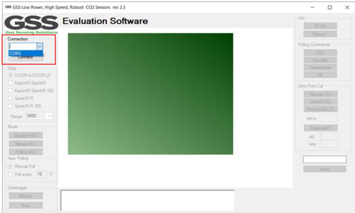
To connect to the sensor, select the correct COM port from the drop-down Connection list, then click the **CONNECT** button. The drop-down list will only show ports with active devices attached.
