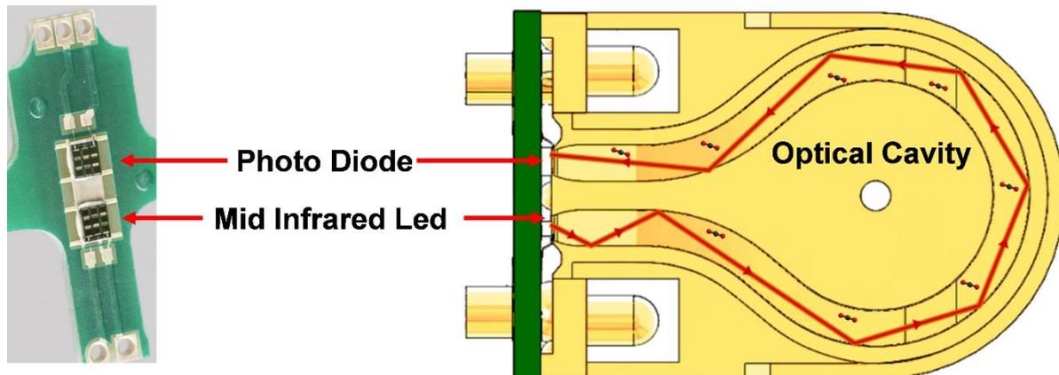
Light from the LED is injected into the optical cavity, which contains the CO<sub>2</sub> gas that has been allowed to enter it through a hole on the top surface. The light that passes through the optical cavity is detected by the photo diode. The signal from the photo diode is digitised by the microcontroller and compared with a reference level stored in memory. The microcontroller can then calculate the level of CO<sub>2</sub> in the optical cavity.
