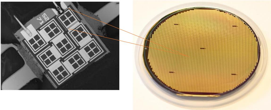
GSS's ultra-efficient LED light source can also be switched on and off rapidly, much faster than conventional incandescent sources. The GSS LEDs can switch on and become usable for CO<sub>2</sub> measurement within seconds. This enables the user to take readings quickly before shutting down the module, thus minimising overall power consumption.
