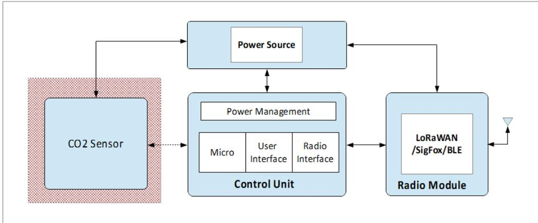
Conventional CO<sub>2</sub> sensors work by illuminating the gas using a filtered incandescent light source and measuring the absorption using a light detector. However, the power consumed using this type of CO<sub>2</sub> sensor is too high to make it usable in a portable, or low power application. The cost of facilities management required to frequently change batteries is impractical and too expensive.
